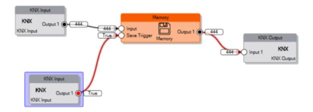
The Memory module is used to store a specific value received at its input and only output it when a trigger condition is met.
