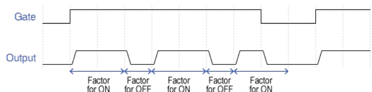
Behaviour of Continuous Pulse Generator
